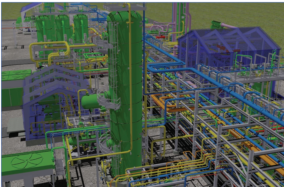
Figure 1. Project review model of Meeker Phase II facility showing the main piperack. In the foreground is the the NGL product amine contactor and behind it are the regeneration gas, dehydration and compression areas. On the right hand side of the main rack is the cryogenic and inlet areas.
