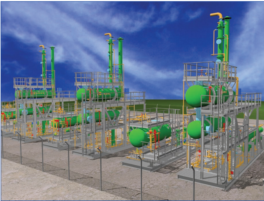
Figure 2. Gas dehydrator plant designed by Gas Liquids Engineering for Industrie Meccaniche Scardellato, Treviso, Italy. The plant was fabricated in Italy, in modular form, and transported to Romania for installation.
